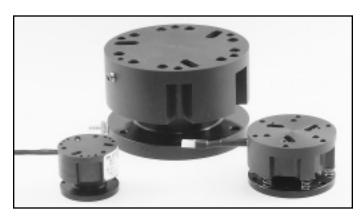
With the exception of Model 4418, all safety joint models are available with either a hard wire or a quick disconnect wire. The quick disconnect feature simplifies the removal of the safety joint from the robot. The molex connector is not recommended for those applications in which the tooling experiences extensive rotary motions.
