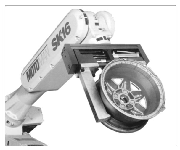
The PX concept was developed for applications that impart high acceleration to heavy objects or require extremely long, precisely positioned jaws. These applications put extreme stress on the gripper. PX grippers use a ceramic bearing system to isolate the precision jaw positioning system from jaw torque and force. The ceramic bearing rail
