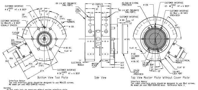
rning: Do not apply lock air pressure without master interface plate properly attached; otherwise, damage may occur to cover plate and o-ring.
